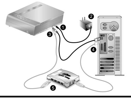
Please make sure the scanner is turned OFFbefore you plug or unplug the scanner powerAttentionadapter.
